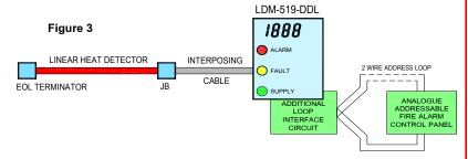
Notes: Configurations for Fig 2 & 3, is dependant on the voltage and current specifications of the LDM-519-DDL being compatible with the monitoring technique and electrical characteristics of the Control Panel / Zone Monitor Unit.
